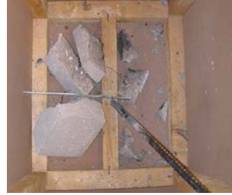
Fig 11: Results after one lightning impulses for specimen D
