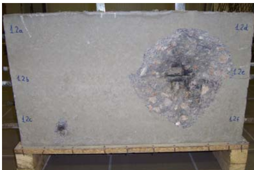
Fig 20: Results after two lightning impulses between 1.1T and 1.2T
