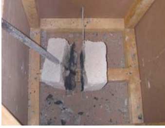
Fig 9: Results after three lightning impulses for specimen B Specimen C was tested third, which had a loose wire to provide an electrical and mechanical connection between the LPS tape and the reinforcement bar. Table 3 summarizes the results, which have proven that specimen C has successfully discharged one lightning impulse with a 10/350 \mu s of 35kA without causing any visual damage to the concrete surface. The second impulse at 57kA has caused an explosion and the concrete was broken.
