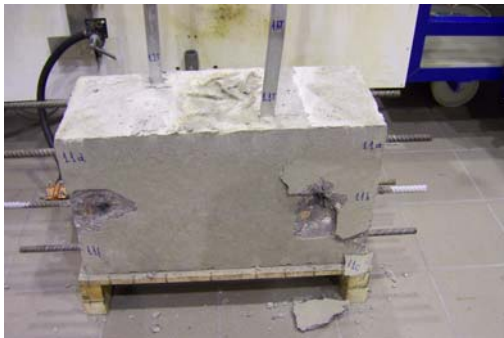
Fig 19: Results after two lightning impulses between 1.1T and 1.2c
