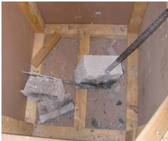
Fig 10: Results after two lightning impulses for specimen C
