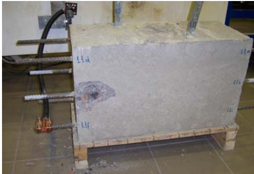
Fig 18: Results after two lightning impulses between 1.1T and 1.1e
